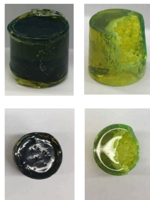
Figure S6. (A) 10g scale cross-linked polymerization flip-experiment with IR lamp; (B) Resulting plastic obtained from IR lamp irradiation (left) and blue lamp irradiation (right).
