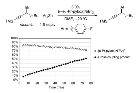
**Figure 9.** Analysis via <sup>19</sup>F NMR spectroscopy of a catalyzed Negishi reaction in progress: (O)  $[(i-Pr-pybox)Ni^{II}Ar]^+$  as a percentage of all nickel that is present; ( $\bullet$ ) yield of cross-coupling product.
