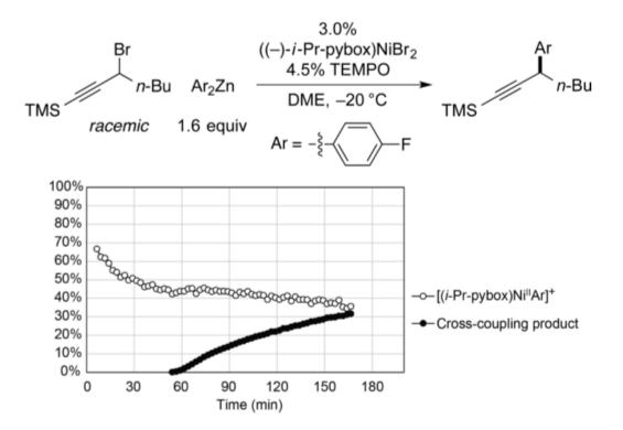
**Figure 11.** Analysis via <sup>19</sup>F NMR spectroscopy of a catalyzed Negishi reaction in progress, in the presence of TEMPO: (O)  $[(i-Pr-pybox)Ni^{II}Ar]^+$  as a percentage of all nickel that is present; ( $\bullet$ ) yield of cross-coupling product.
