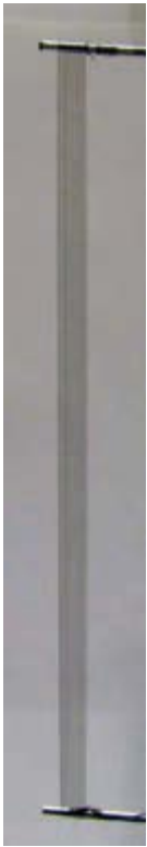
50-mm-long 2-mm-wide nanotube aerogel sheet
