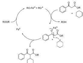
Scheme 4. Tentative mechanism for the Fe-catalyzed alkylation with simple alkanes.
