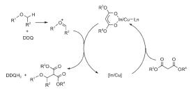
$<sup>\</sup>ensuremath{\textit{Scheme 3.}}$  Possible mechanism for the CDC reaction of ether with malonate.
