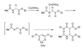
*Scheme 2.* Proposed mechanism for the oxidative functionalization of glycine derivatives with diethyl malonate.
