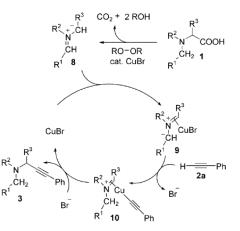
Scheme 3. Proposed mechanism for the copper-catalyzed decarboxylative coupling between an  $\alpha\text{-}amino$  acid and phenylacetylene.
