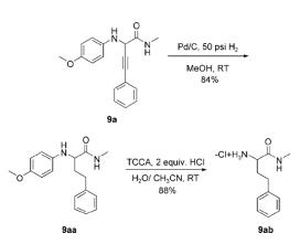
*Scheme 4.* Synthesis of homophenylalanine derivative **9ab**. TCCA=Trichloroisocyanuric acid
