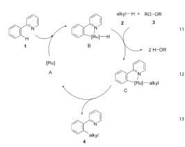
Scheme 2. Proposed mechanism for the ruthenium-catalyzed cycloalkylation of arenes mediated with peroxides.
