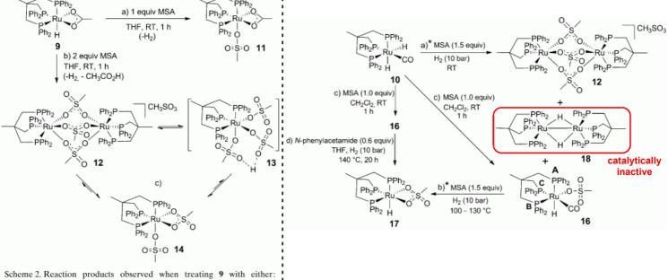
Scheme 2. Reaction products observed when treating **9** with either a) 1 equiv, or b) 2 equiv of MSA.
