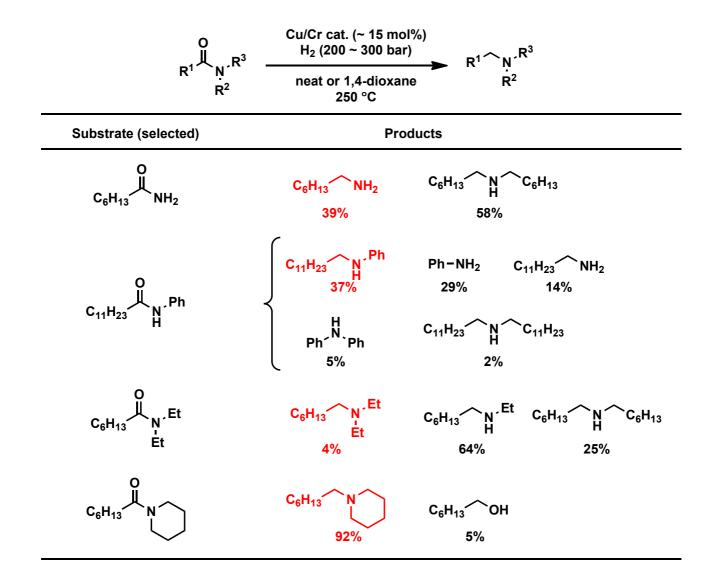
• Extremely high H<sub>2</sub> pressure (~ 300 bar) and reaction temperature (250 °C) were required.
