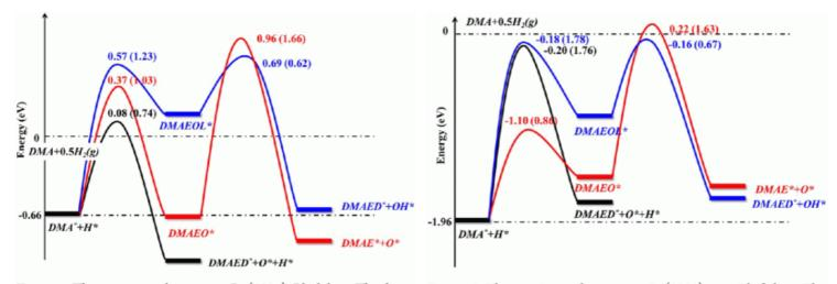
**Figure 4.** The reaction pathways over Ru(0001). Black line: The direct cleavage pathway. Blue line: O-H activation pathway. Red line: C-H activation pathway. The stabilities of the TSs with respect to absorbed DMA and H are listed (eV) and the energy barriers of the corresponding elementary steps are listed in parentheses (eV).
