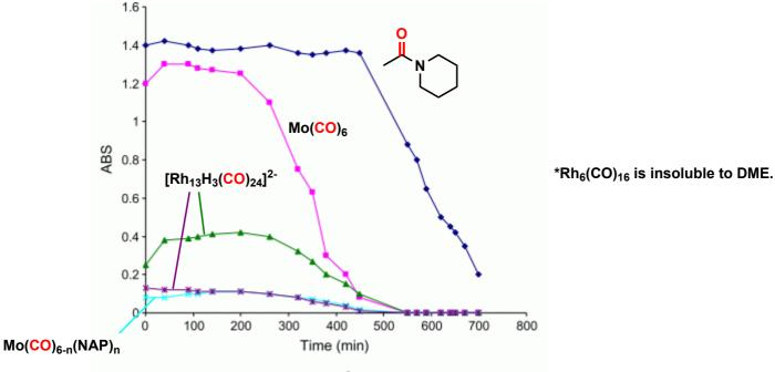
**Fig. 2.** In situ HPFTIR spectra (2100–1600 cm<sup>-1</sup>) showing decay and disappearance of v(CO) absorptions during catalyst genesis and initiation of hydrogenation. Key: **NAP** (1658 cm<sup>-1</sup>), **MO**(CO)<sub>6</sub> (1984 cm<sup>-1</sup>), **2016** cm<sup>-1</sup>,  $\times$  1849 cm<sup>-1</sup>,  $\times$  1752 cm<sup>-1</sup>.
