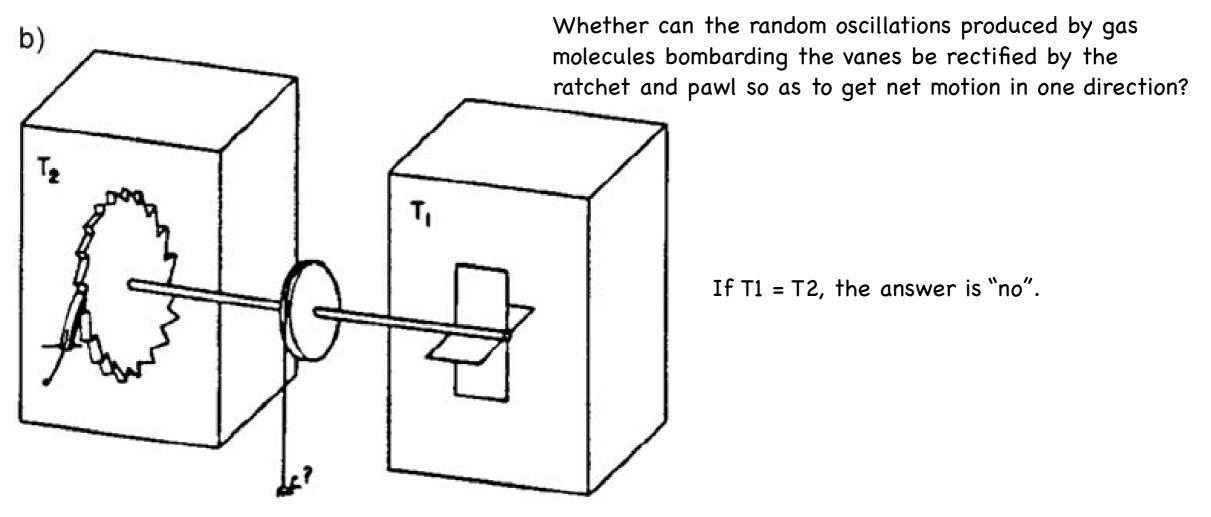
However, on the contrary, cooling the ratchet and pawl by external means makes it possible to rectify the random motion.
