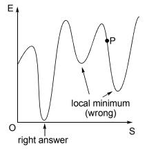
Simulated Annealing algorithm in pseudo-code Select an initial state  $i \in S$ ; Select an initial temperature T > 0; Set temperature change counter t = 0; Repeat Set repetition counter n = 0; Repeat Generate state j, a neighbour of i; Calculate  $\delta = f(j) - f(i);$ If  $\delta < 0$  then i := jelse if random $(0, 1) < \exp(-\delta/T)$  then i := j; (A) n := n + 1: until n = N(t); t := t + 1;T := T(t);until stopping criterion true.
